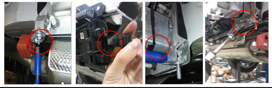
$\underline{4}$ . Trim the impact bars mounting plate by 1" (See Figure 4). Repeat this process from the opposite side.
