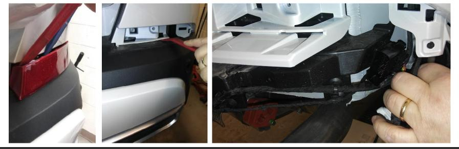
2. Lower exhaust and disconnect sensor wiring: Use a 13mm socket to remove 2 nuts from the exhaust (1 each side). Next disconnect the back-up sensor wiring and hands free sensor (Not shown). Lower tailgate to access upper mounting fasteners.
